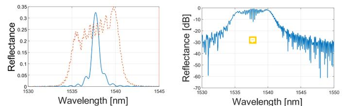
Fig.4 Reflectance for second case. On the left: linear reflectance of the first grating (solid line) and linear reflectance of the second grating (dashed line). On the right: reflectance of FP resonator in logarithmic scale.
