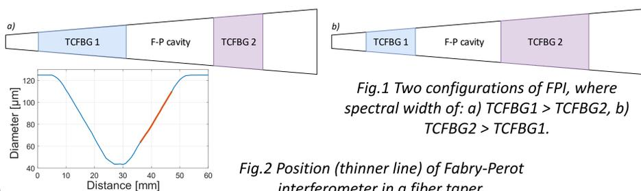
Fig.1 Two configurations of FPI, where spectral width of: a) TCFBG1 > TCFBG2, b) TCFBG2 > TCFBG1.
