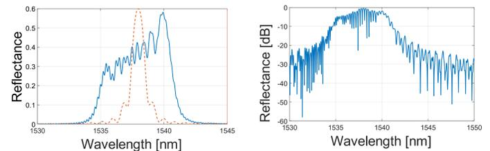
Fig.3 Reflectance for first case. On the left: linear reflectance of the first grating (solid line) and linear reflectance of the second grating (dashed line). On the right: reflectance of FP resonator in logarithmic scale.
